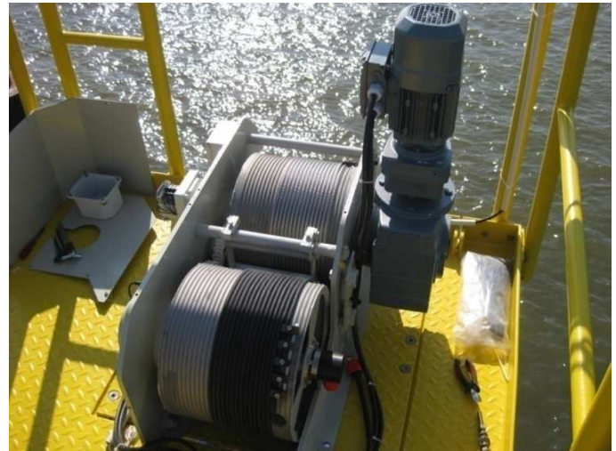
Fig. 3: Winch at the Platform to move the Slide on the Chain Guide
