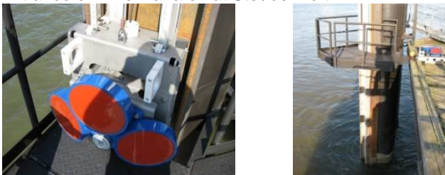
Fig. 2: Vertical Slide (left) and Pile with mounted Chain Guide of the HADCP (right)
