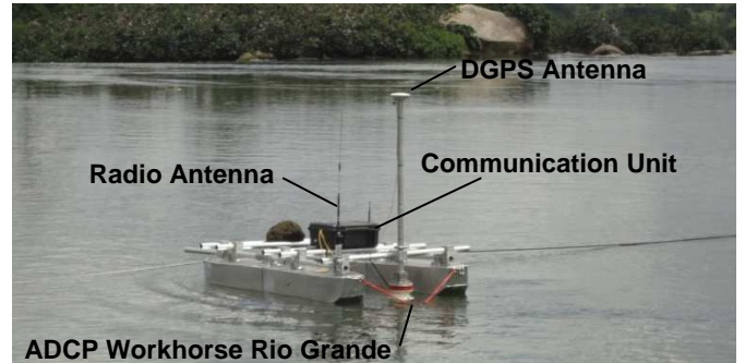
Fig. 3: Pontoon with ADCP and Communication Unit
